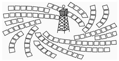
Tiny florets in a sunflower's center are arranged in an interlocking spiral, which inspired engineers in the design of this solar power plant. Mirrors positioned at the same angle as the florets bounce light toward the power plant's central tower.
